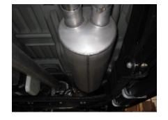
3. Install muffler #B onto head pipe 1.5" to 2" muffler should be level use clamp #E to secure together do not tighten.
