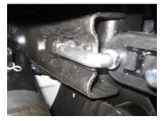
5.Next install drivers side rear hanger and grommet with bolt kit provided. See picture the hanger goes on the outside of the frame and bolts through the first wall of the frame.
